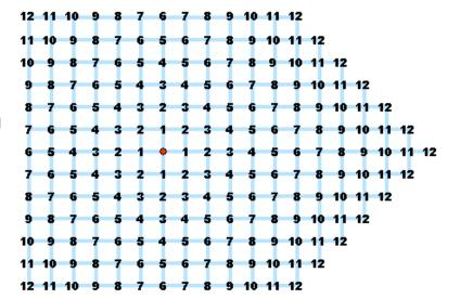
The molten plastic cannot flow through the fly swatter holes, so distance must be calculated by moving horizontally and vertically. If a single injection site (the red dot) is used for the head of the fly swatter the molten plastic must travel 12 cm to get to all the corners (see above). A good choice for a set of injection points doesn't allow any point to get too far away from an injection site.
